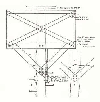
Figure 54. Detail from plans for the Tree Development Observatory, 1933. Designed for use on the Kootenai National Forest, Montana and Clearwater National Forest, Idaho.
